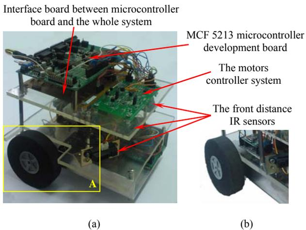
Figure 1. (a). Robot prototype; (b) detail of the previous implementation [12]
